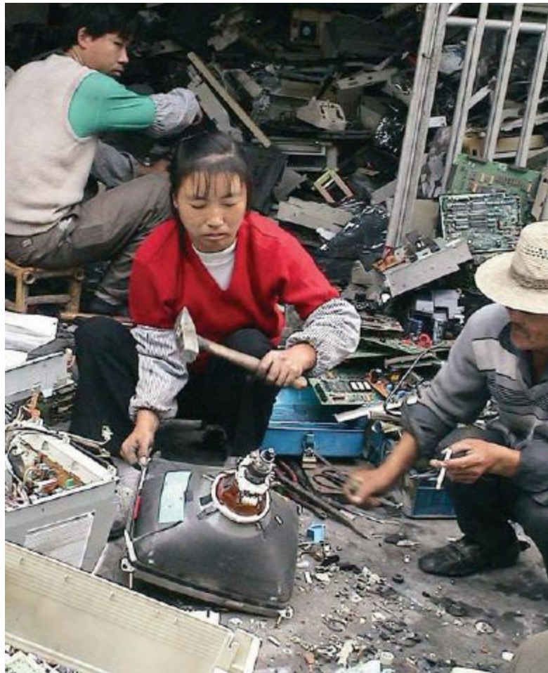
In a makeshift recycling center, a Chinese woman uses a hammer to open an old cathode ray tube. She wants the copper that is inside, but in the process she will release several pounds of lead into the soil and groundwater. Scientists have found alarmingly high levels of toxic heavy metals in the rivers that flow by such rural recycling operations.
