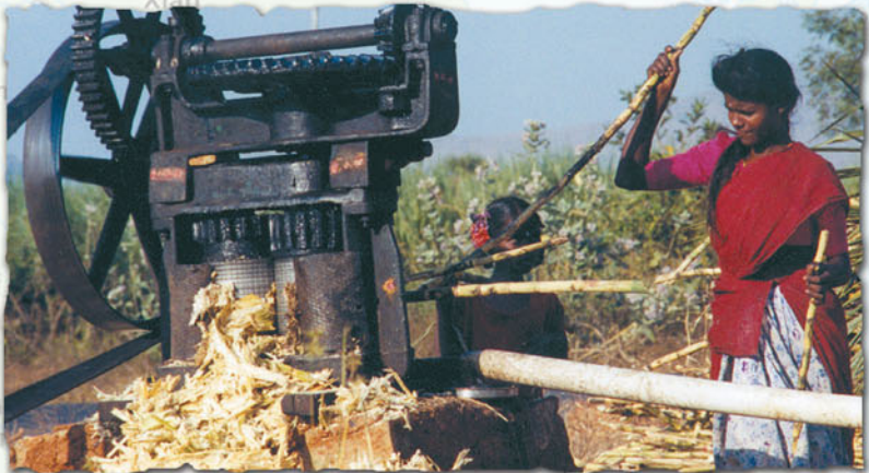
When I saw this unusual sight, I had to stop and talk to the workers. From historical pictures, I knew that belt-driven machines were common on U.S. farms 100 years ago. This one in Tamil Nadu processes sugar cane. The woman feeds sugar cane into the machine, which disgorges the stalks on one side and sugar cane juice on the other.
